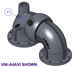
AVIATION SPECIFIC SWIVELS (WITH AVI SUFFIX) USE GREASE SPECIFICALLY FOR AVIATION APPLICATIONS AND HAVE THE GREASE NIPPLE REPLACED WITH A ST STEEL GRUBSCREW TO AVOID STANDARD GREASE BEING INJECTED DURING REGULAR MAINTENANCE
